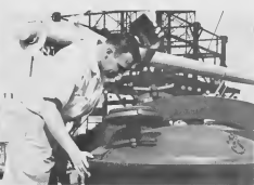
USING A mirror to reflect the sun's rays, Commander Jackaway inspects ship's tanks for dryness and cleanliness. This prevents product contamination from previous cargoes.
